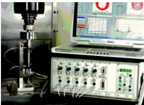
Figure 3 The spindle for a CNC Vertical Machining Center with variable speed, AC motor and angular contact, ball bearing spindle. The five probes are configured in a stiff nest for measuring motions of a two-sphere target rotating in the spindle. The probes will measure the total of: “Bearing error motion,” “structural error motion,” “target eccentricity” and “target non-roundness.” Boring a hole with this spindle would be an example of a rotating sensitive direction.
