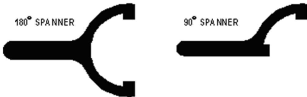
When installing tapered bore bearings that utilize an adapter sleeve and locknut, a spanner wrench is used to complete the assembly and set the clearance. A spanner is a specialized wrench with a series of pins or tabs around the circumference. These pins or tabs fit into the notches of a locknut. The 90° spanner is the most common; however the 180° spanner requires less effort since all of the force applied at the handle is translated to torque on the nut.
