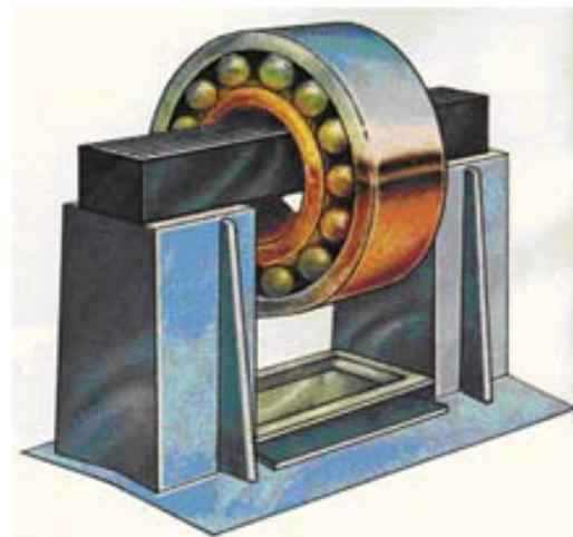
Small and medium size bearings with interference fit inner rings are commonly mounted with the aid of a bearing heater. The purpose of the bearing heater is to expand the inner ring enough so that the bearing can be slipped on the shaft, up to the shoulder without the use of force. Bearing heaters have many advantages but can also destroy a bearing very quickly. Bearings heaters should be equipped with certain safe guards to prevent permanent bearing damage.
