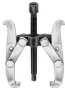
When it becomes necessary to remove a bearing from an assembly, care must be taken to avoid damage to raceways and rolling elements. In these instances, utilize a bearing puller. There is wide variety of sizes, capacities and styles from which to choose.
