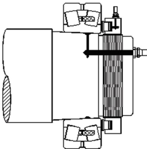
The installation of large diameter bearings often requires the use of hydraulics for mounting and removal. This makes the job easy and fast and eliminates the huge physical effort needed to do the job. Hydraulics are commonly used for tapered bore bearings and occasionally for cylindrical bore bearings.
